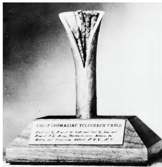
Figure 2: 1846: The World's First Armoured Submarine Cable, Samuel Colt (N.Y.)
