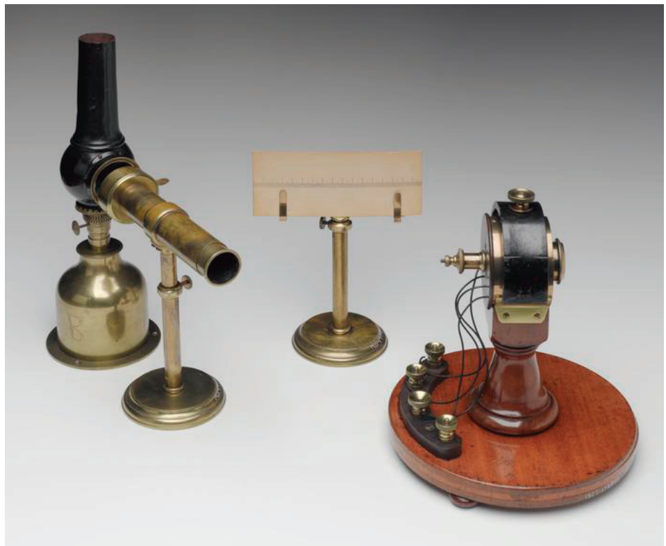
Figure 6: 1857: “Optically Amplified” Submarine Terminal
