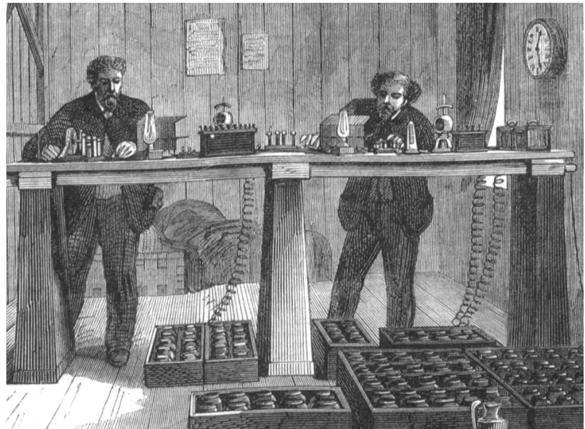
Figure 7: 1865 Atlantic Cable Station Ireland: Two submarine line terminals each with a Mirror "Galvo" and Lanterns
